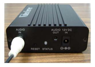
If user needs not only video stream but also audio stream, then the audio source should be attached to Video Server. User may utilize line output of standard camera or audio amplifier, or others as the audio source. Connect the RCA terminal of audio device's line output to the Video Server's RCA input and make sure to power on your camera or audio device first.
