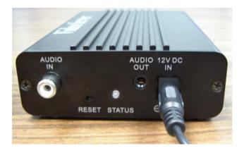
Connect the external power supply to the 12VDC power in connector of the Video Server. Note: Use the power adapter, 12VDC, included in the package and connect the other end to wall outlet for AC power.
