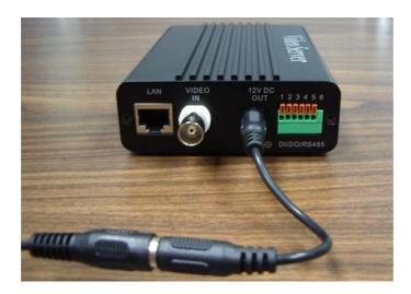
The Video Server can provide 12VDC out to supply one external camera. **Note** that the output current is 400mA maximum.
