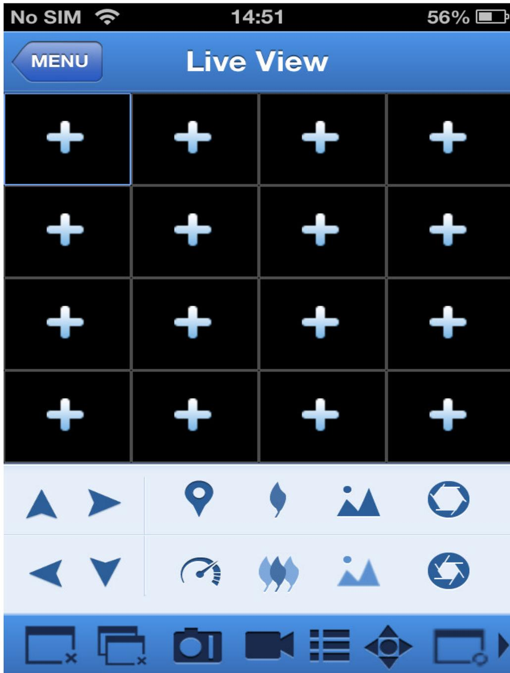
You need to Maximize a camera window and open PTZ mode to control the camera. Tab Arrows on the side of camera window to control camera move side to side or up and down. And other control buttons allow you to do Zoom, Force, Iris, PTZ speed and Preset, etc. As shown in the follow figures.
