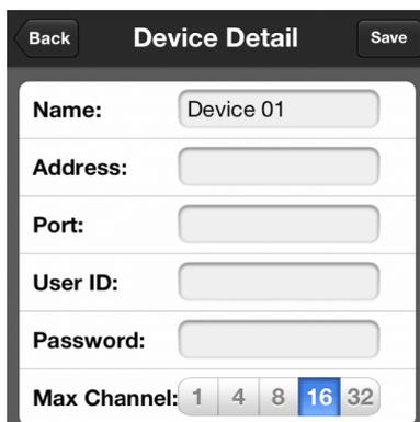
**Name:** It is the name of the monitoring equipment, which will help you identify the device easily;
